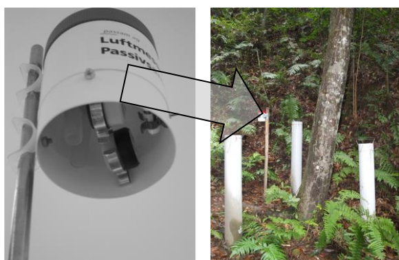
Protective shelter for ammonia and forest measuring site
